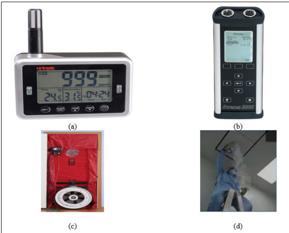
Figure 1. Example device (a) Rotronic CL11 device, (b) Swema3000, (c) Blower door, (d) Smoke
